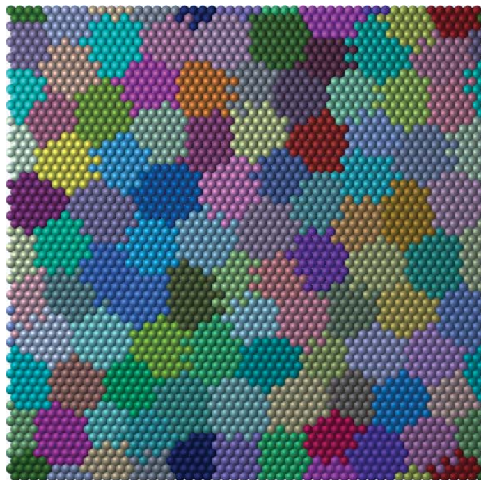
Figure K2: A depiction of a partition of a 2D LJ triangular lattice with periodic boundary conditions. The corresponding multiresolution plot is in Fig. K1 where the small peak on the left occurs at \gamma \simeq 39 . This peak indicates the largest natural clusters for this particular lattice system.
