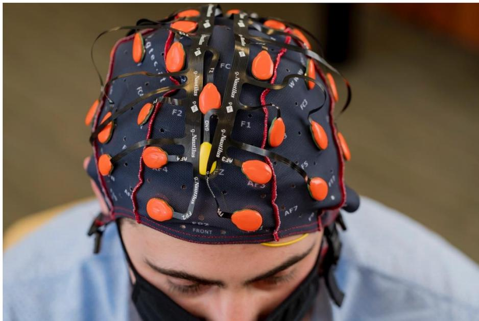
Figure 2: The EEG Device On the Scalp
