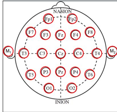
Figure 1: 10-20 Assignment of the Scalp EEG Device [15]
