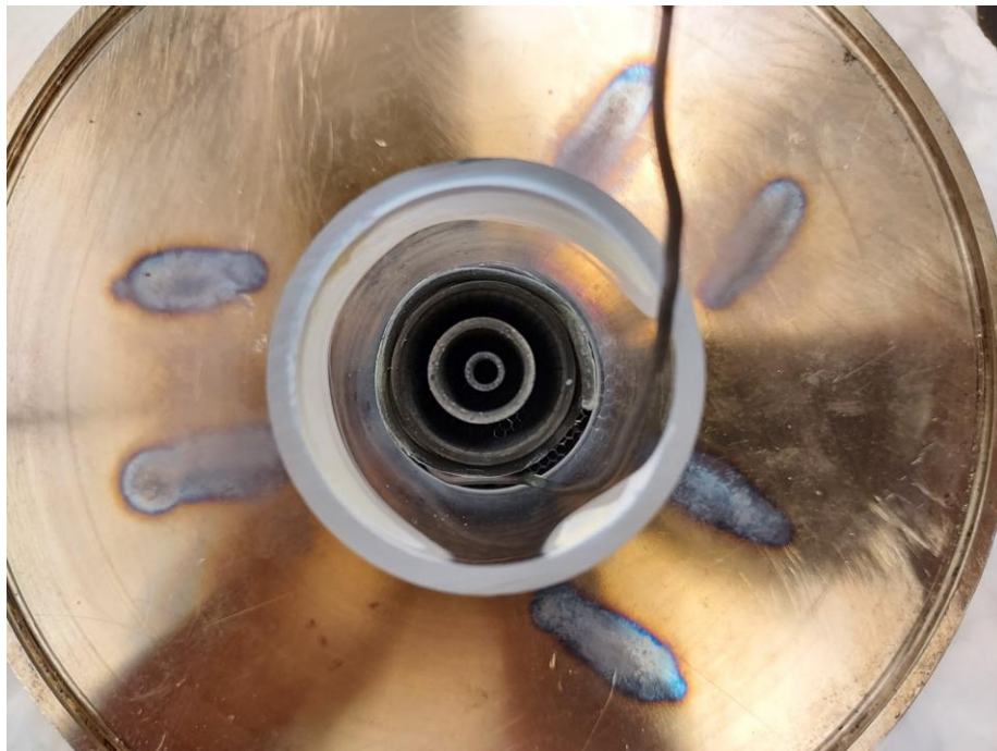
Fig. C.3. Top view of the FLAME burner without the nozzle and vacuum chamber.
