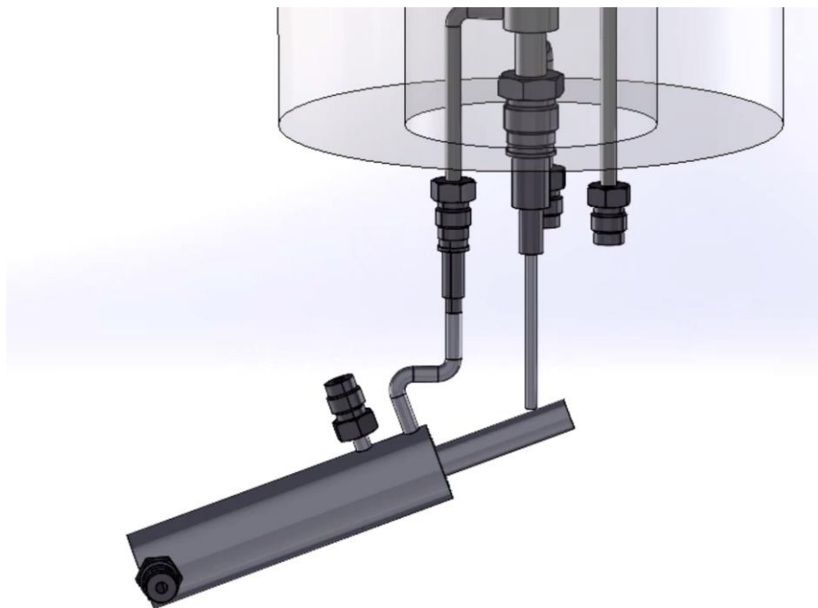
Fig. C.6. 3D model view of the sodium vaporizer.
