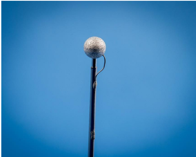
Fig. B.5. Closeup of the porous spherical burner and burner surface thermocouple prior to launch to the ISS.
