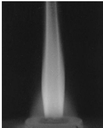
Fig. 8.2. Photo of a TiCl_4 -Na-Ar flame producing salt-encapsulated, pure Ti particles. Reproduced from [199].
