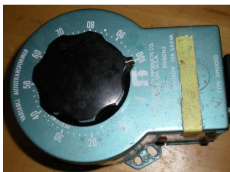
Figure 6.2: Variable AC controller used for adjustment of the spinning speed.
