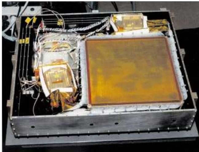
Figure 2.1: The Cosmic Ray Isotope Spectrometer (CRIS). The large, gold-colored square is the top of the SOFT hodoscope (Section 2.2). Other visible elements include the high-voltage power supplies, the image intensifier/CCD system, and the camera electronics.
