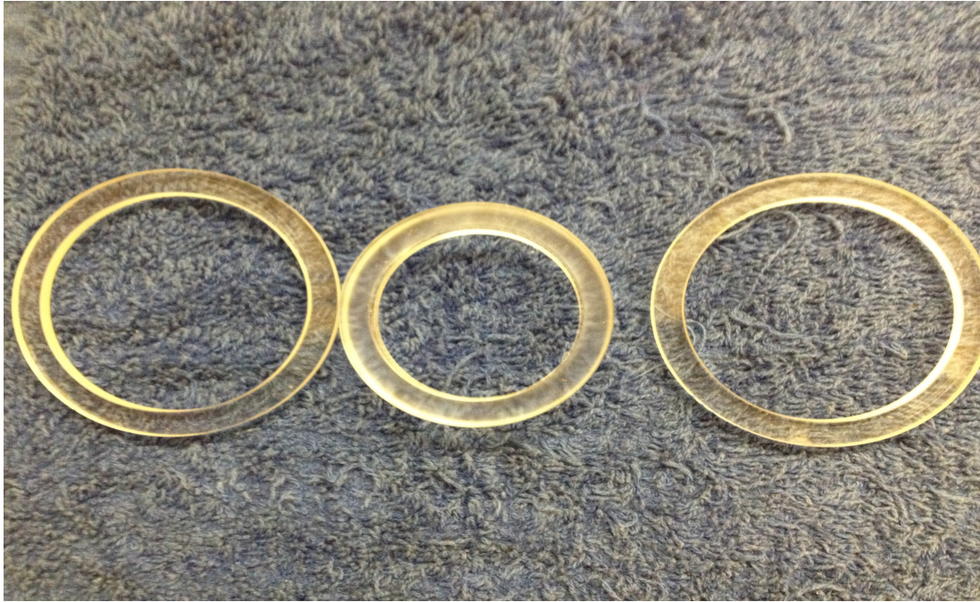
FIGURE 3.6: The disassembled sample mold showing the three main pieces. Photography by Ben Johnson.
