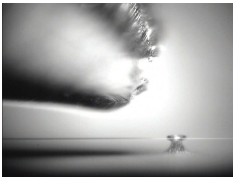
Figure 3.8: Microscopic image showing the microtoroid and the nozzle used to deposit nanoparticles.
