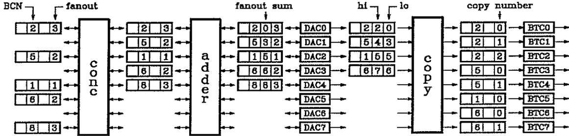
Figure 2: Example of Operation of Lee's Multicast Architecture
