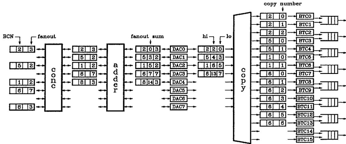
Figure 3: Example of System with Expanding Copy Network
