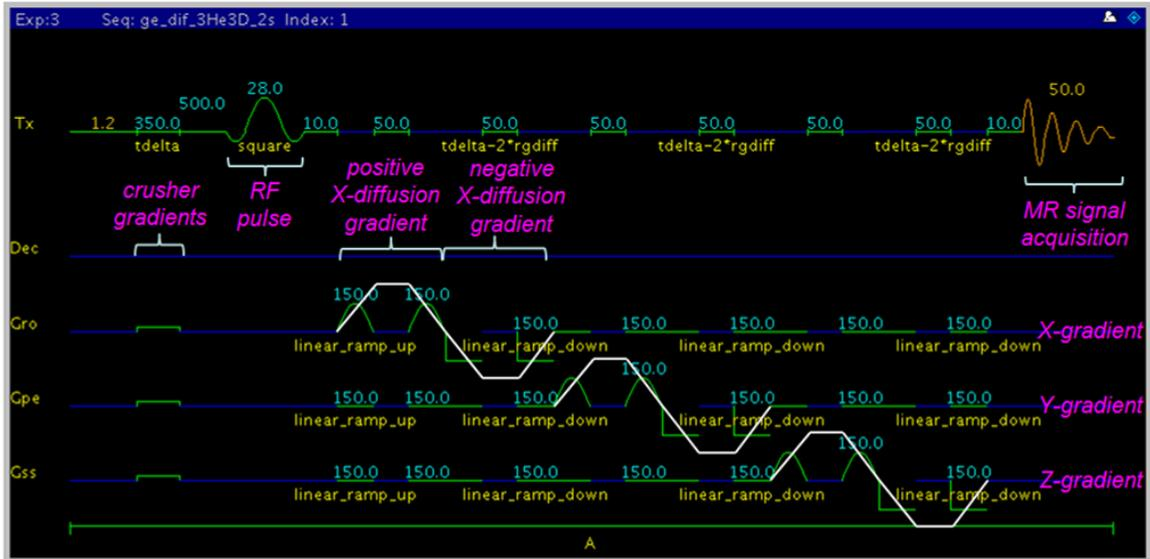
**Figure 6.3:** The X, Y, Z diffusion sensitizing gradient sequence used in all anisotropy MR experiments. The sequence utilized the descending set of b-values,  $b[s/cm^2]=0, 4, 3, 2, 1, 0$ . The purple italics denote the main sequence parts: crusher gradients followed by the RF pulse and all three consecutive bi-polar gradients, X, Y and Z.
