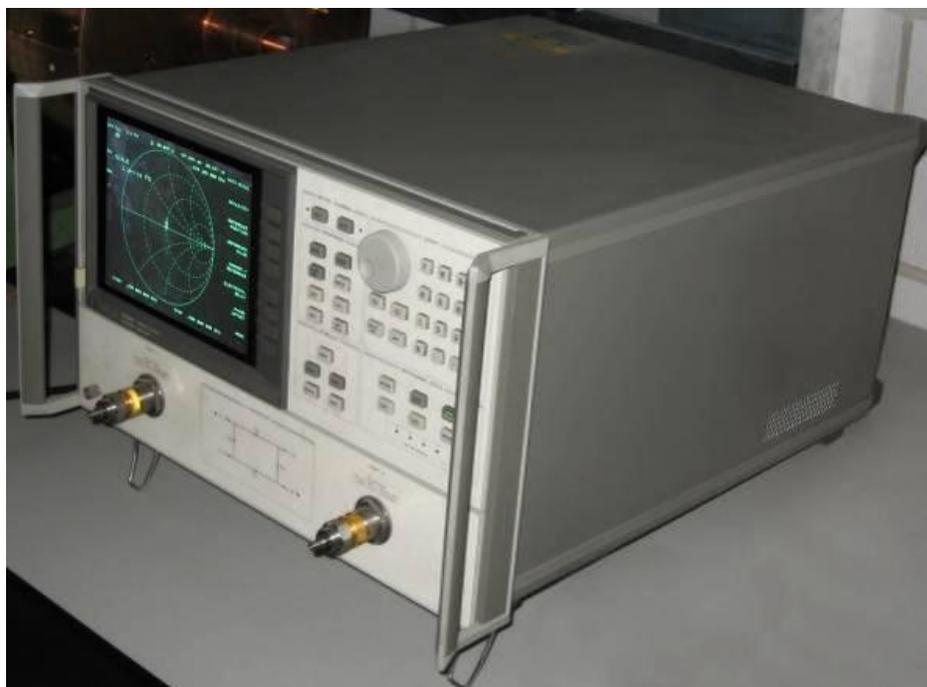
**Figure 5.13:** Network Analyzer, HP 8720A, used to tune the RF coil to the  $^3\text{He}$  nuclei frequency and to adjust the inductive coupling, with the load present in the coil.
