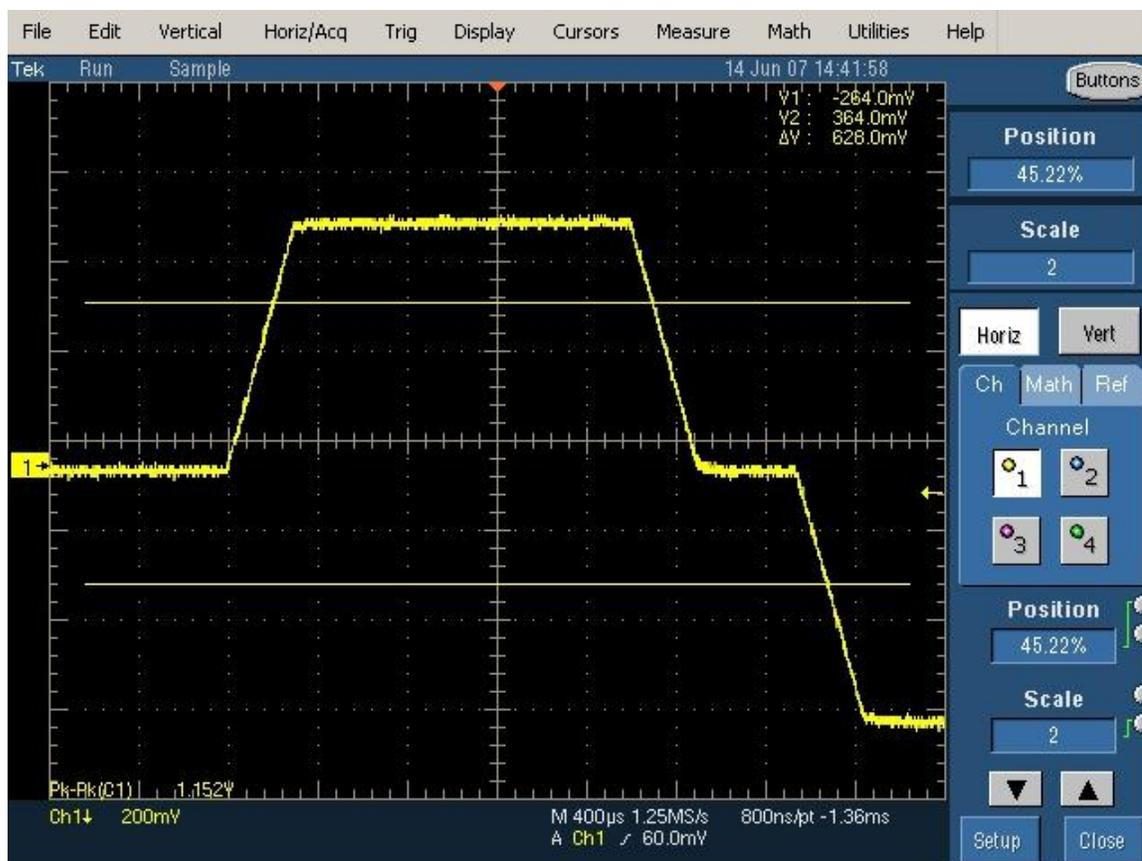
**Figure 5.5:** The bi-polar gradient transition region behaves well: gradient follows the prescribed waveform for both, positive and negative side. The gradient moves through the transition points without ringing or soft corners, allowing us to apply the mathematical theory for the gas diffusion in lungs with the required accuracy and confidence in results.
