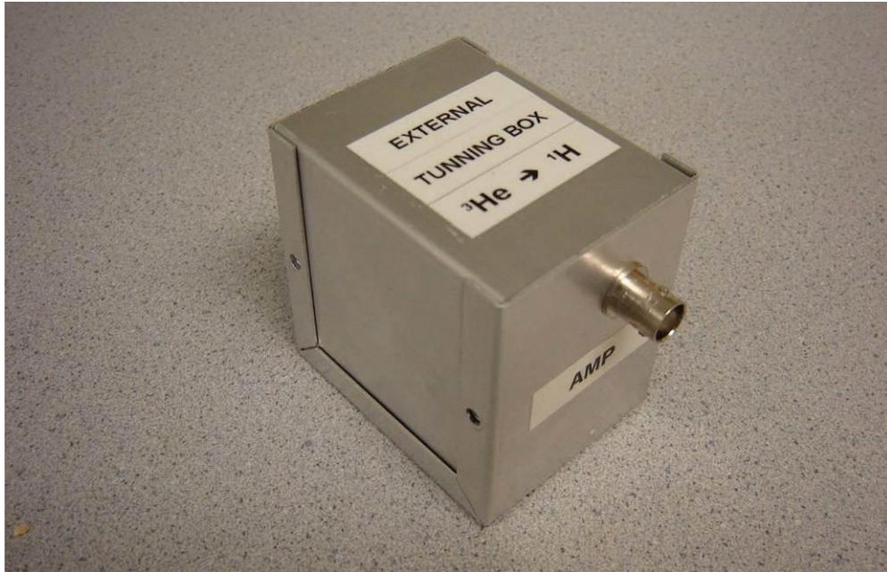
**Figure 5.6:** External tuning box, consisting of one inductor and two capacitors, one fixed one adjustable. The adjustable capacitor is there to tune the box to the right resonance, in this case the frequency of proton ( $^1\text{H}$ ).
