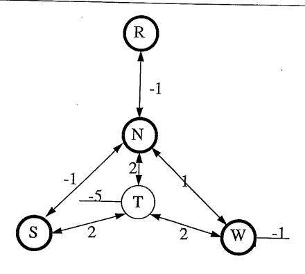
Figure 1: A symmetric network that represents the function E = -2NT - 2ST - 2WT + 5T + NS + RN - WN + W, describing the WFF:  $(N \land S \to W) \land (R \to (\neg N)) \land (N \lor (\neg W))$ . T is a hidden unit.
