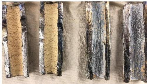
**Figure 2-1: Pipes sections with scales (left 1&2), pipe sections after scales were scraped off (right 1&2)**
