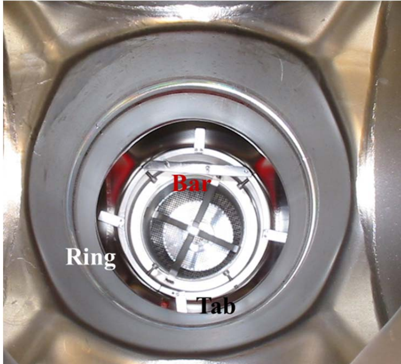
Figure A1.3 Photograph of sample guide ring inserted into the chamber.
