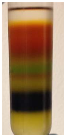
Figure 4.2 Sucrose gradient ultracentrifugation for the PscA-PscB purification. The dark green band in the middle of the gradient contains the PscA-PscB complex
