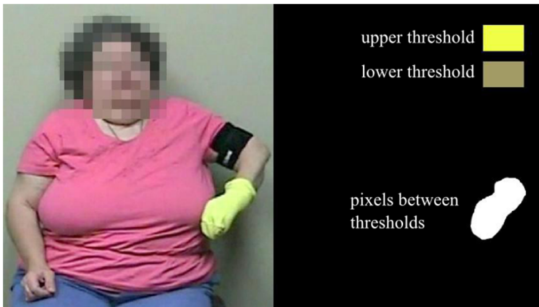
Figure 2.7. Segmenting the tracked object using HSV color thresholds.
