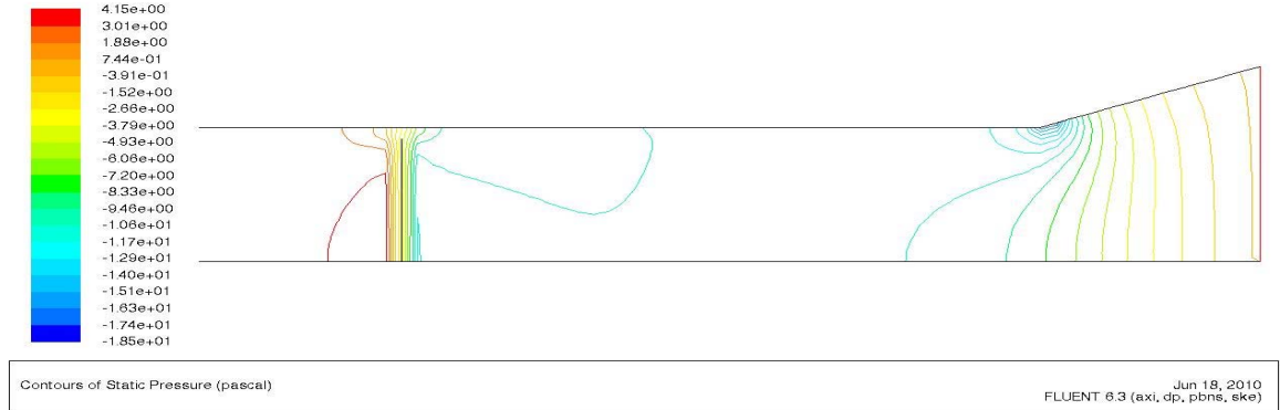
Figure 3.6 Zoomed-in-View of computational domain for flow inside the silo enclosing the turbine with a diffuser on the top: static pressure contours and their magnitude. The silo has been rotated by 90deg. clockwise in this figure.
