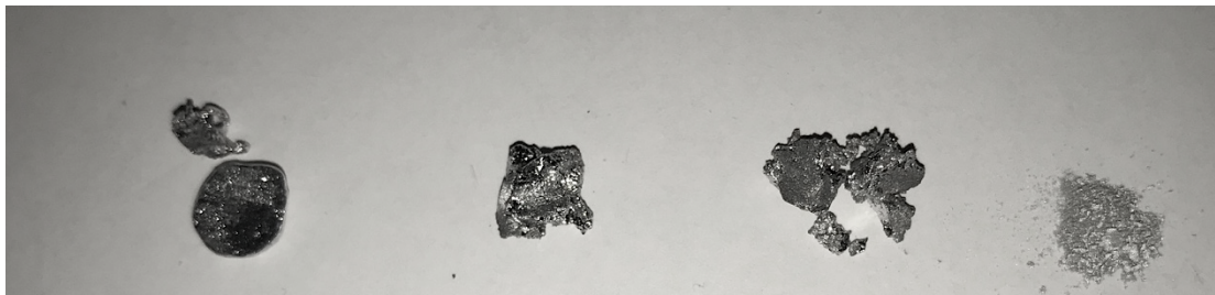
Figure 9. Four composite samples with paraffin concentrations of 21.8%, 40.3%, 50.1%, and 61.2%, from left to right. The 61.2% sample was almost granular due to the high concentration of paraffin.
