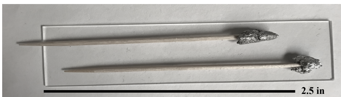
Figure 10. Two fabricated composite samples 21.83% (top) and 40.32 (bottom) affixed to toothpicks and are resting on a glass slide. Within the micro-CT testing chamber, each sample was positioned with the sample end of the toothpick uppermost and analyzed individually.
