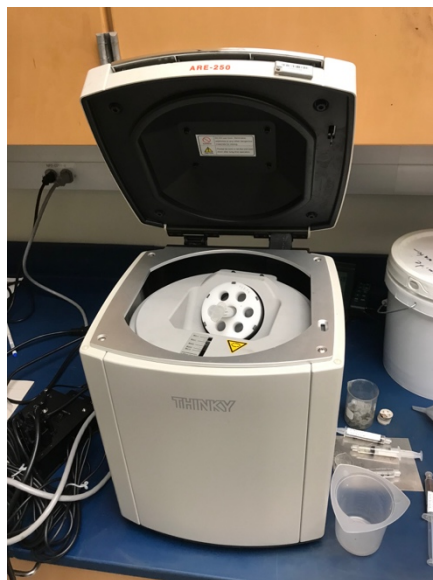
Figure 7. The Thinky ARE-250 mixing and degassing machine.
