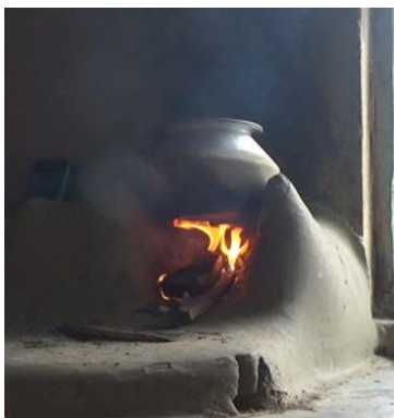
Figure 4.1: Traditional one-pot mud chulha used in this work.
