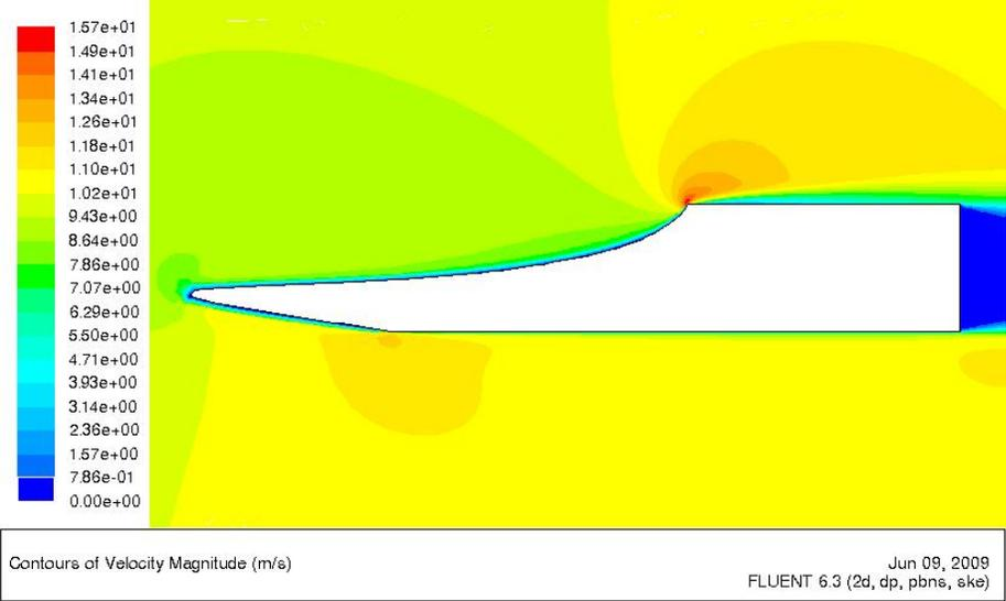
Figure 4.28 Velocity contours for Case 5  $C_d$ -optimized truck front,  $Re_H = 303,957$
