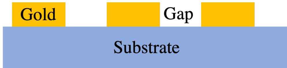
Figure 7.1: The section of a typical mask. The gold is deposited onto the surface of some substrate.
