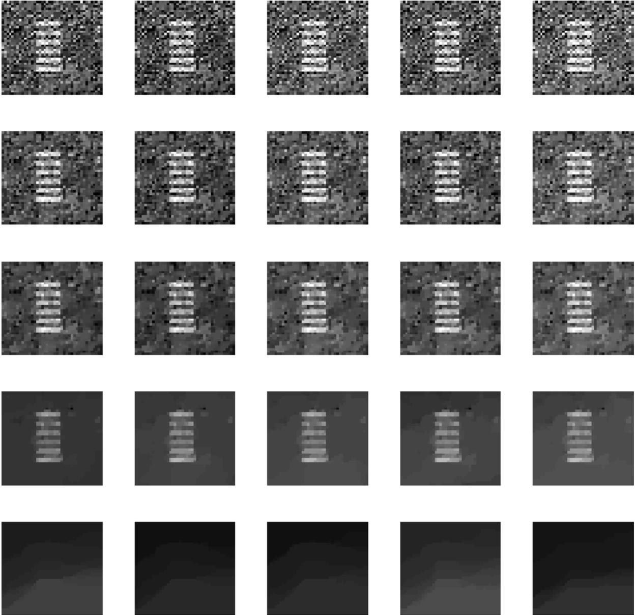
Figure 5.11: The bar region of the reconstructed  $\delta$  image of the analytical geometric phantom for the AAP ( $2\pi$ ) design with the different regularization parameters specified in Table 5.1. From left to right, the regularization parameter for  $\beta$  is increasing. From top to bottom, the regularization parameter for  $\delta$  is increasing.
