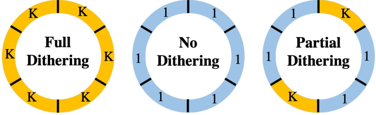
Figure 6.2: A comparison between no-dithering, full-dithering and partial-dithering when  $V = 6$  and  $D = 3$ . Each arc represents a tomographic view angle. The numbers on the arcs orange arcs denote the number of exposures taken at the view angle. The orange arc means  $K$ -step dithering is implemented at the view angle, while a blue arc means there is only 1 exposure taken.
