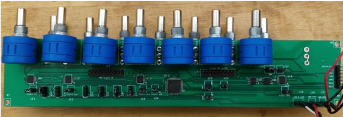
Figure 2. 5 PMT gain controller provides different gains to each PMT through control software
