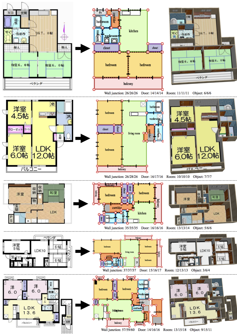
Figure 4.4: Floorplan vectorization results. From left to right, an input floorplan image, reconstructed vector-graphics representation visualized by our custom renderer, and the corresponding popup 3D model. We have manually checked the correctness of each junction and primitive estimation, whose statistics are shown under each example.
