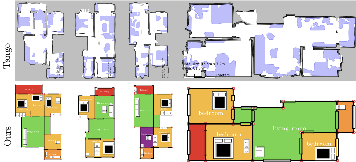
Figure 5.7: Comparison against a commercial floorplan generator, Tango Navigator App. Top: Floorplan image from Tango. Bottom: Our results.
