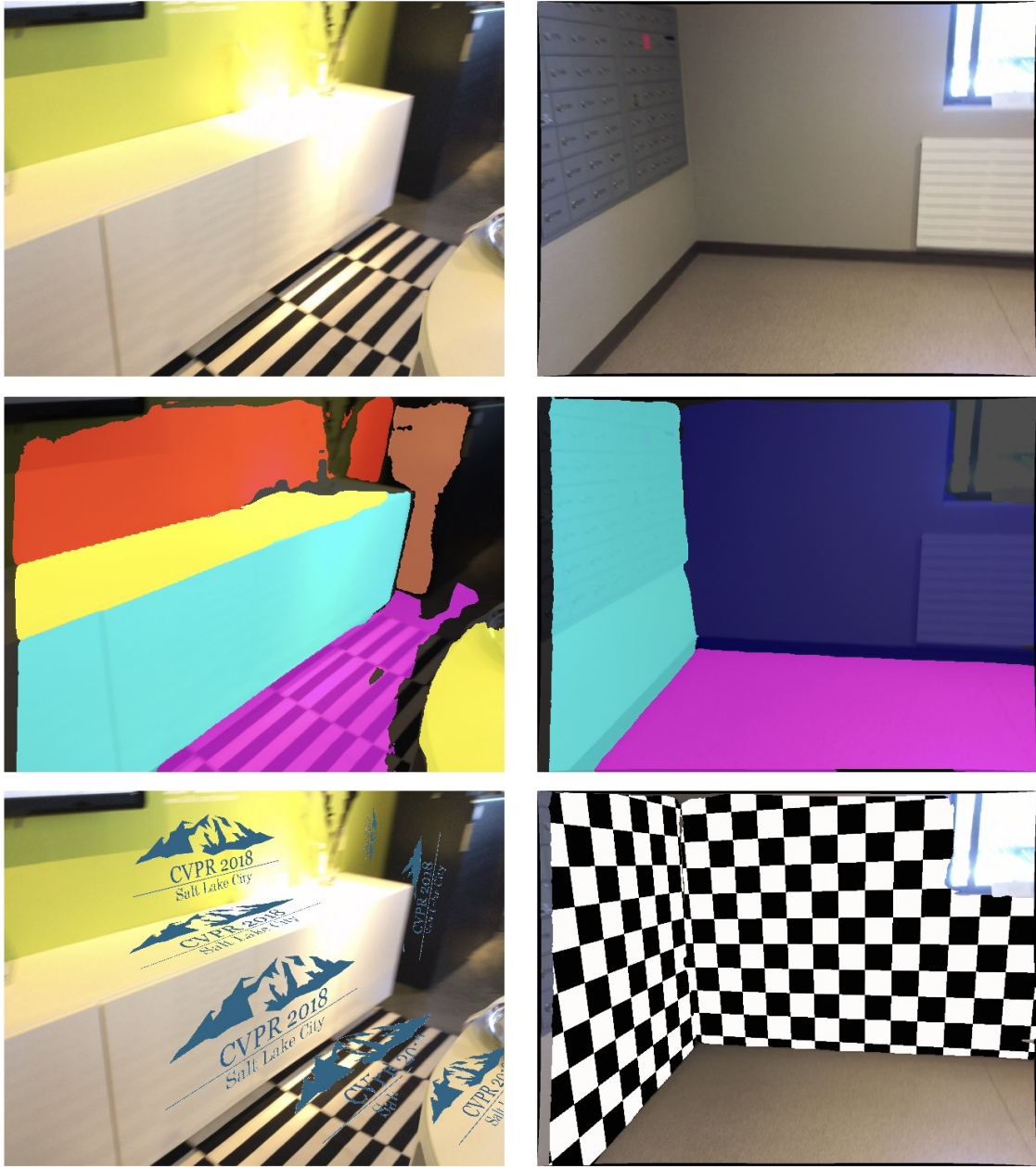
Figure 2.7: Texture editing applications. From top to bottom, an input image, a plane segmentation result, and an edited image.
