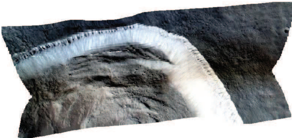
Figure 3.8: Results with different penalties for CRISM FRT0001DC22 on Mars in Fig 3.7. Reconstructions are shown in RGB with wavelengths 0.71 \mu\text{m} , 0.599 \mu\text{m} and 0.534 \mu\text{m} . Frames are \sim 10 \text{ km} across. Note the row artifacts in Fig. 3.8a is corresponding to the sensitivity mapping in Fig 3.7.
