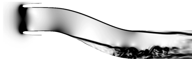
Figure 1.2 Navier-Stokes DES modeling flow separation in an s-duct diffuser [2]
