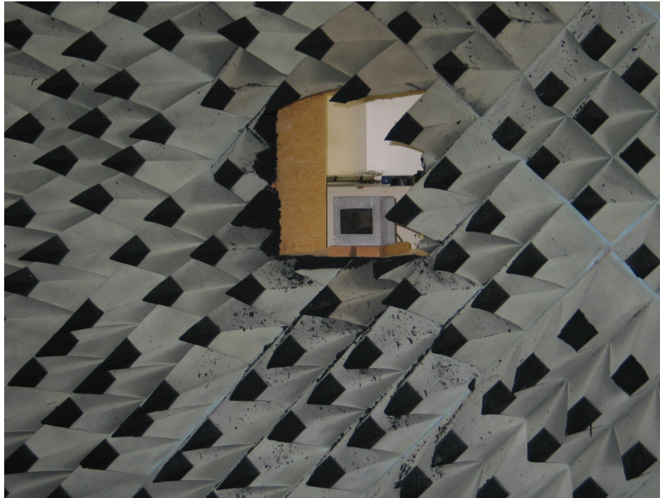
Figure 33: Receiver View of the Anechoic Chamber
