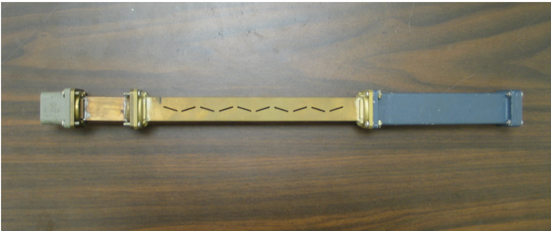
Figure 28: Leaky Wave Antenna with Excitation and Matched Load
