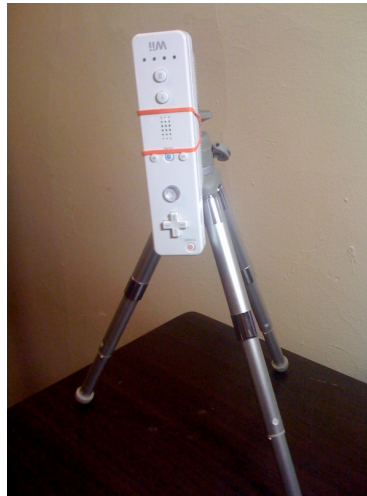
Figure 3.1 Wii Remote on tripod for IR tracking
