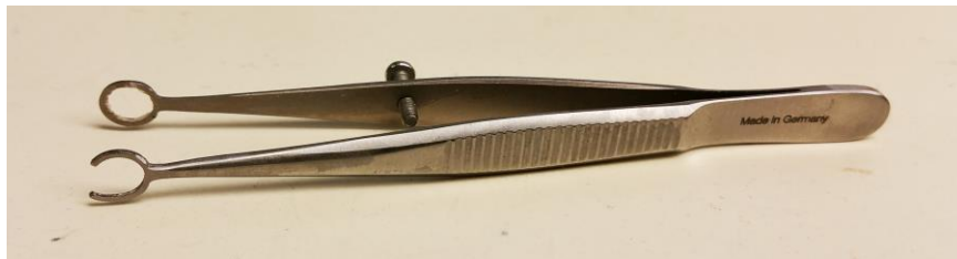
Figure 6.32 Modified ring forceps. Ring forceps with a hole ground out of one of the rings.
