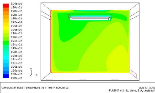
Figure 5.59 Temperature contours in yz-plane at z-50 after 7.5 minutes (vents open -flow on)
