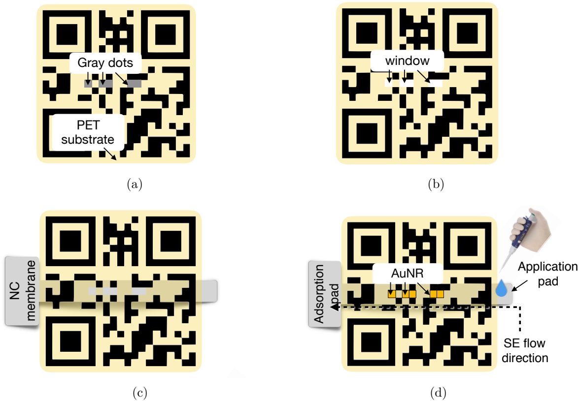
Figure 4.12: Illustration of QR code FEC biosensor fabrication procedure: (a) QR code printed on the mesoporous substrate using normal ink; (b) The plastic substrate in the gray colored square dots area removed; (c) NC membrane is attached on the back side of the QR code; (d) AuNR ink is printed on the yellow area.
