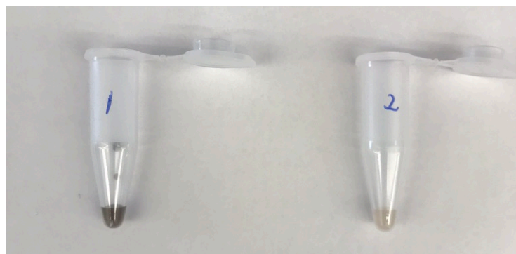
Figure A.7: Black color in tube 1 is due to reaction between dopamine and \text{AgNO}_3 which is consumed by \text{Cl}^- (due to PBS) to generate \text{AgCl} in tube 2.
