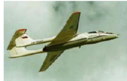
M-55 stratospheric aircraft (Geoscan Network) Piloted aircraft for the delivery of wireless services and remote sensing
