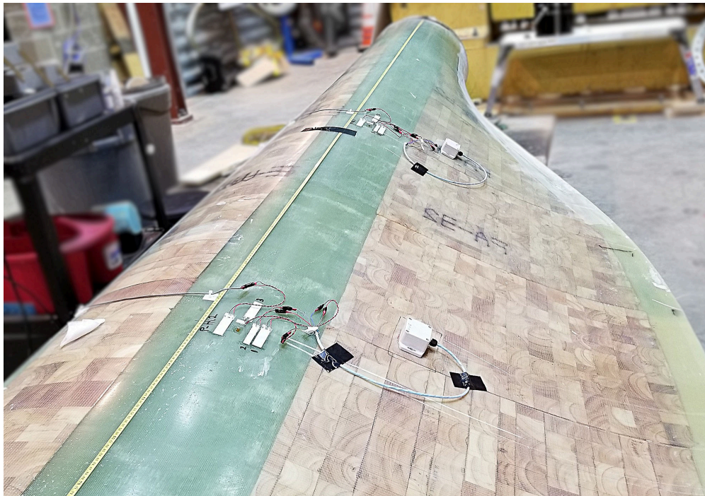
Figure 6.30: Sensor boxes on a wind turbine blade that was tested in collaboration with NREL.
