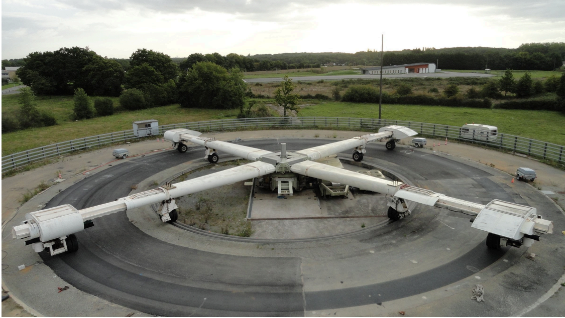
Figure 6.17: The BioRePavation test facility, coordinated by IFSTTAR, in Nantes, France.
