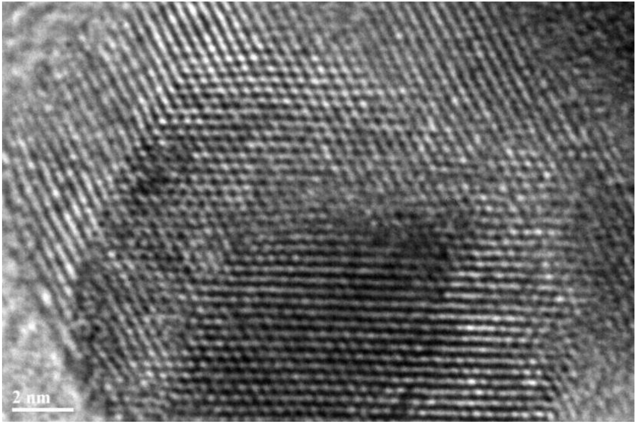
Fig. 5.2: TEM micrograph of nickel-coated YSZ powder (2nm scale)
