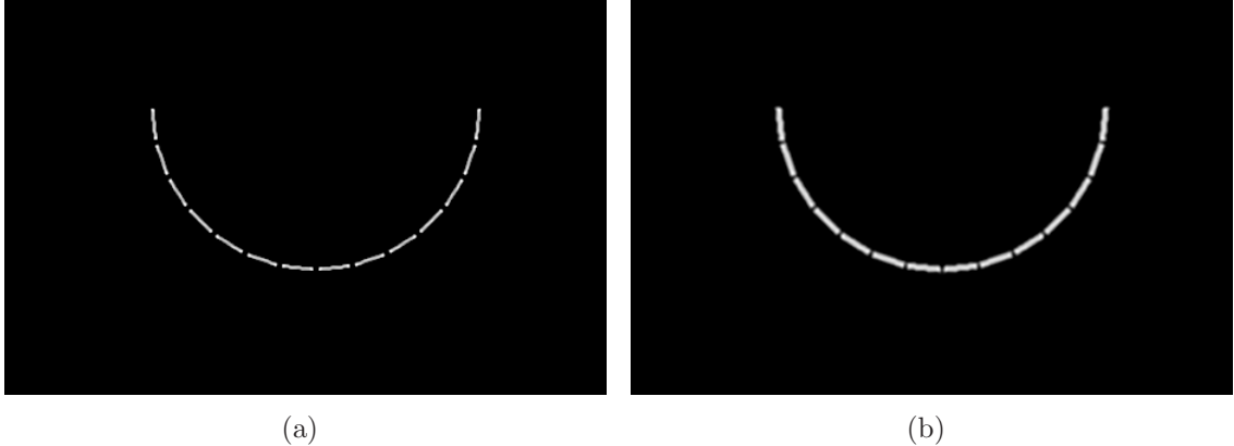
Figure 6.10: Reconstructions of the analytically-simulated water half-ring transmission scan. (a) Window min/max = [0.0075, 0.0115] \text{mm}^{-1} ; (b) window min/max = [0.0, 0.012] \text{mm}^{-1} .
