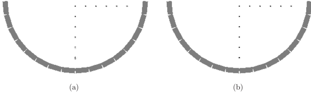
Figure 5.8: II+IS+SS reconstructions of point sources using (a) non-DOI insert crystals; (b) 4-layer DOI insert crystals. The insert blocks have been overlaid on the reconstructed images for reference.
