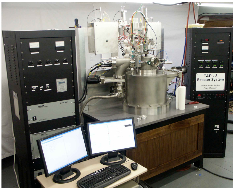
Figure 3.2 TAP-3 Reactor System.
