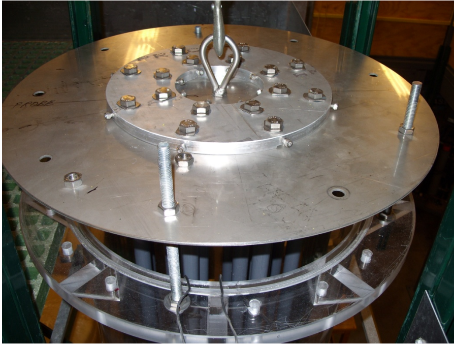
Fig. B.3 – Top plate hooked to top crane.
