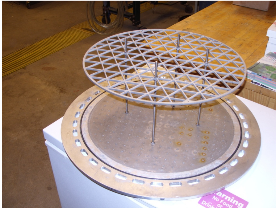
Fig. B.2 – Lower spacer for 25% internals attached to distributor
