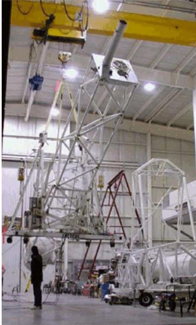
Figure 3.1. InFOCUS balloon gondola. The X-Calibur polarimeter will be located in the focal plane of the Wolter X-ray mirror (40 cm diameter) with a focal length of 8 m [72, 73].
