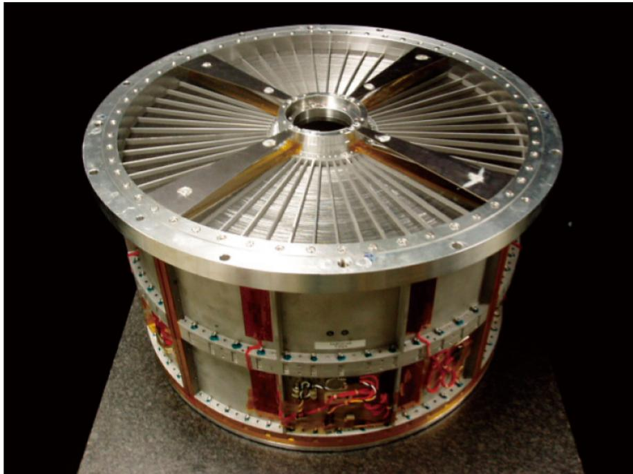
Figure 3.2. The InFOC $\mu$ S Al-mirror assembly. It comprises 255 double reflection shells, each made of 0.17 mm thick Al-foils with a multilayer coating for a broad energy range [72, 73].
