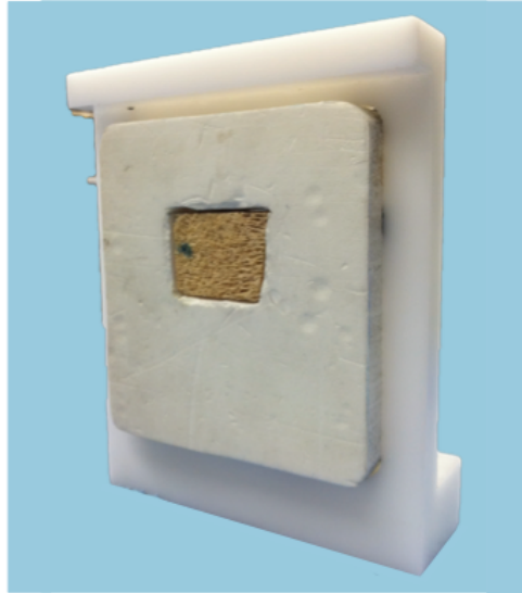
FIGURE 4.2: Sample holder consisting of a custom-cut piece of high density styrofoam fit into a Delrin frame. The Delrin frame was attached to a computer-controlled motion controller. Photograph by Amber Groopman.
