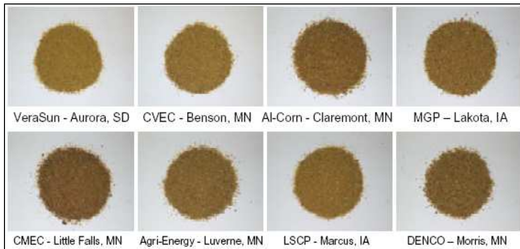
Figure 1.5: DDGS samples from various US ethanol plants, showing that color variation is significant from plant to plant
