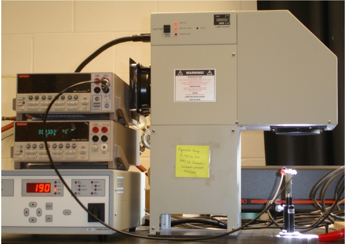
Figure I-5: Digital image of the solar simulator used for photovoltaic testing in Chapter 7.
