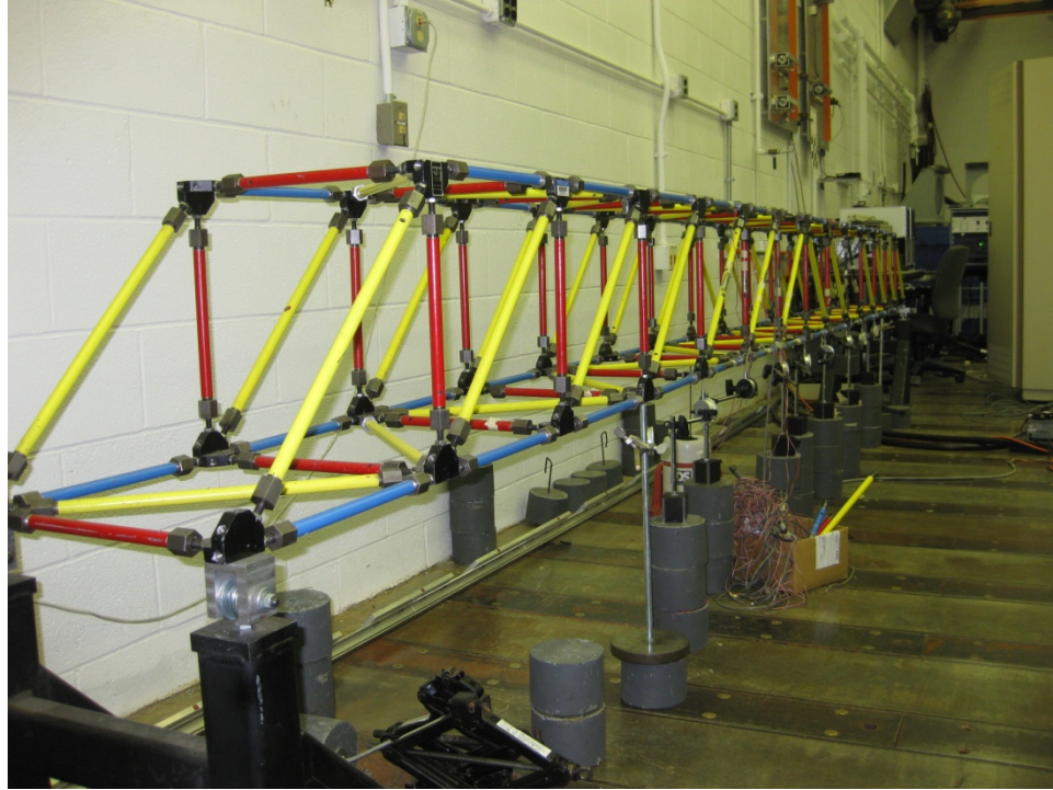
Figure 6.1 Fourteen Bay Three Dimensional Truss Test Structure in the Smart Structures Technology Laboratory at the University of Illinois Urbana-Champaign
