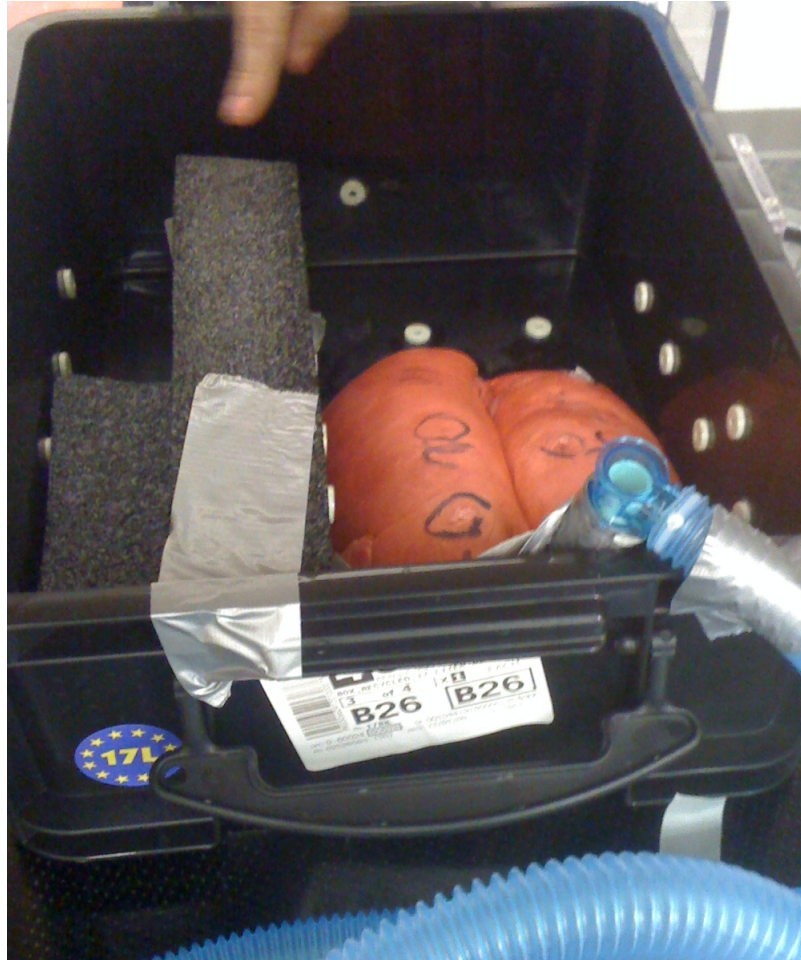
Figure 5.10: Porcine Lungs. The lungs were affixed in a housing which maximized the amount of anterior/posterior and superior/inferior motion by restricting the lateral edges. The lungs were attached to ventilator and inflated via positive pressure.
