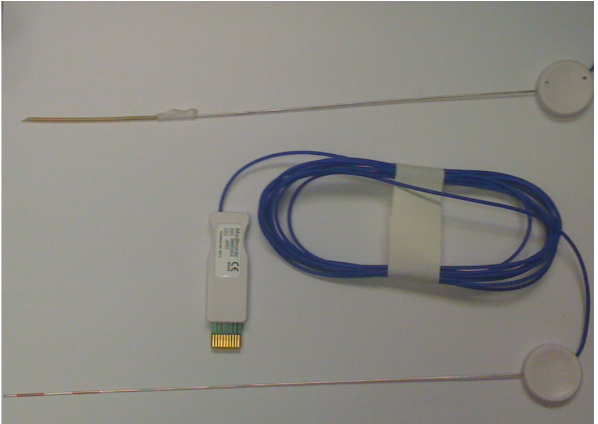
Figure 5.11: Surgical tools. An AxiEM stylette with PEEK guide sheath/needle as well as a bare AxiEM stylette are shown.
