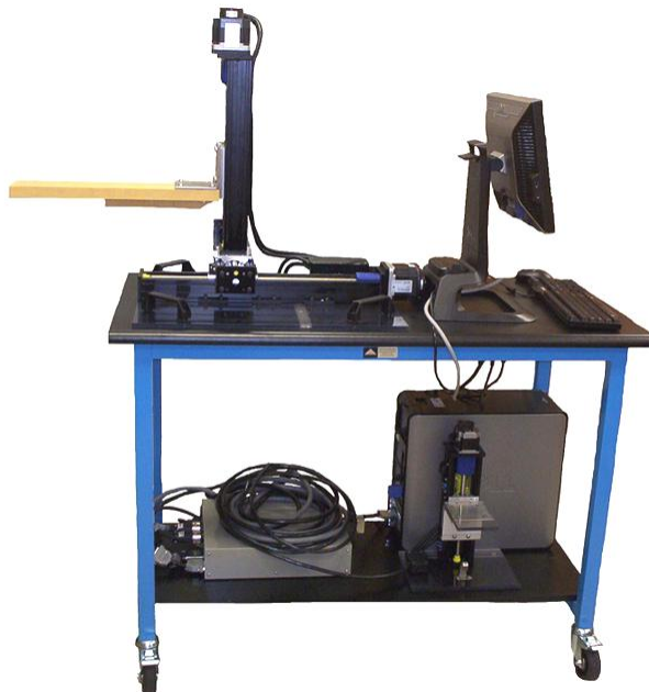
Figure B.1: The Washington University 4D Phantom.
