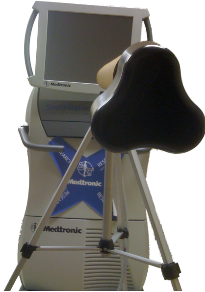
Figure 5.1: Medtronic StealthStation. The field generator (black, foreground) and the Medtronic StealthStation (background) are shown. A position sensitive magnetic field is generated with respect to the field generator, which allows for precise location monitoring of EM tools in the tracking volume.
