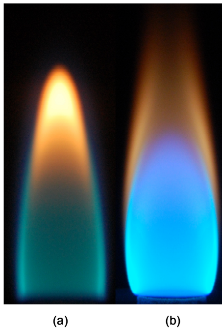
Figure 4.2. Photographs of (a) normal and (b) inverse sooting limit flames. The sooting limit is observed at a height of 8 mm from the burner tip.
