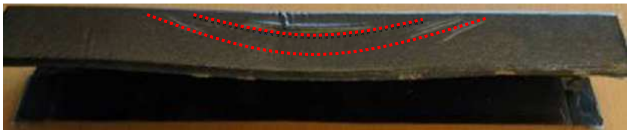
Figure 14: Common Off-Angle Wrinkles of Joggled C-Channel (adapted) [1]
