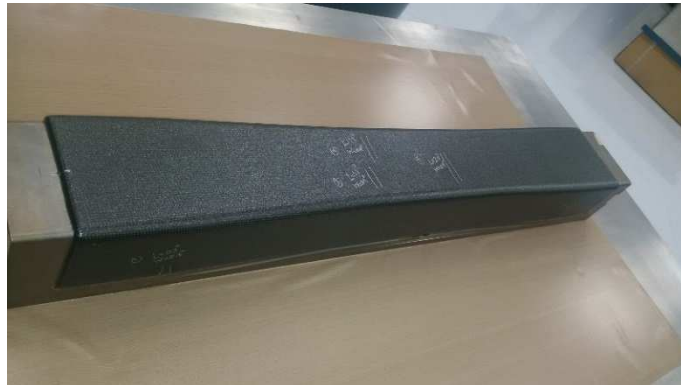
Figure 51: Typical PW Wrinkles
