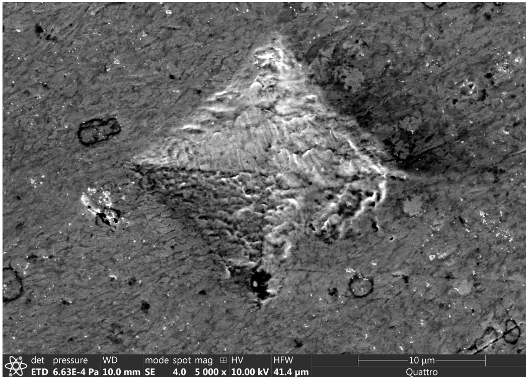
Figure 3 SEM secondary electron image showing a Vickers indent and microstructure on Row 4. Scale bar reads 10 \mu m.
