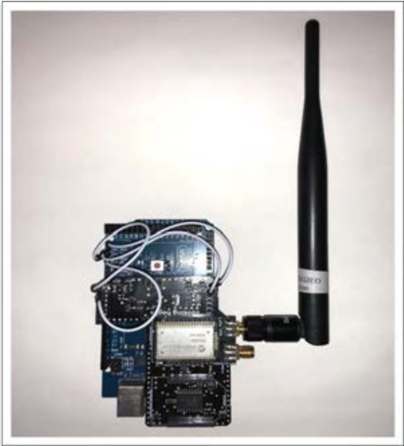
Figure 6.2: Arduino MEGA, Connection Bridge, & Cooking Hacks LoRaWAN Module Setup
