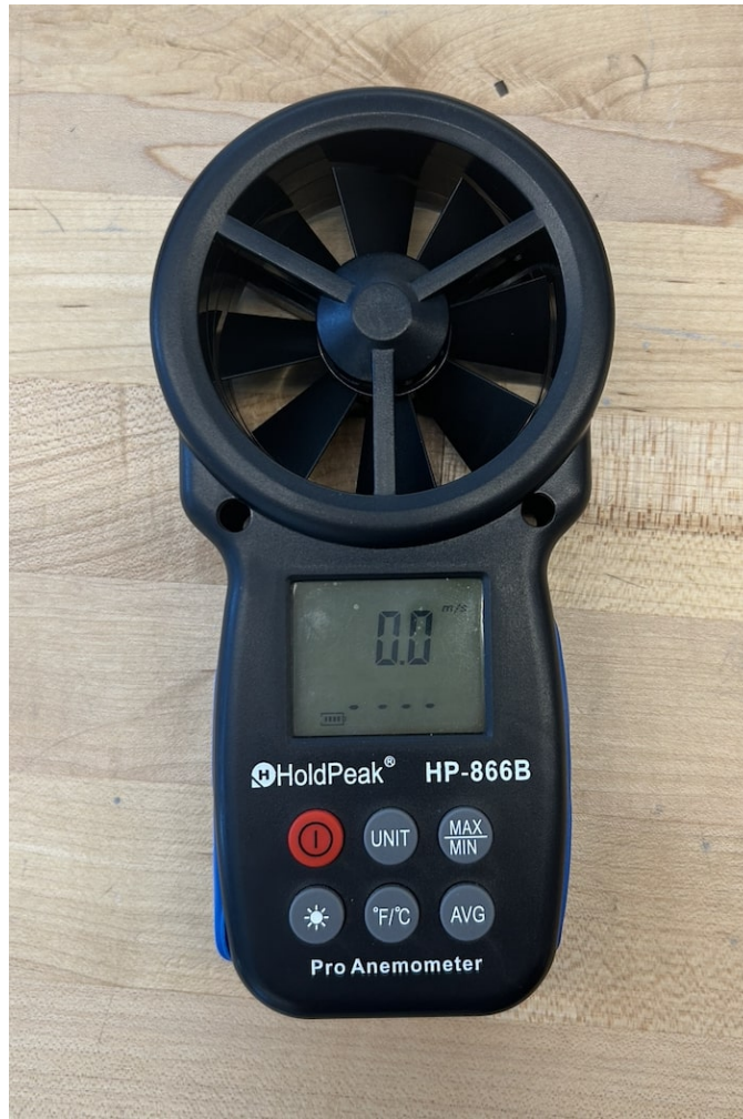
Figure 21: HP-866B Anemometer used to find wind speeds.
