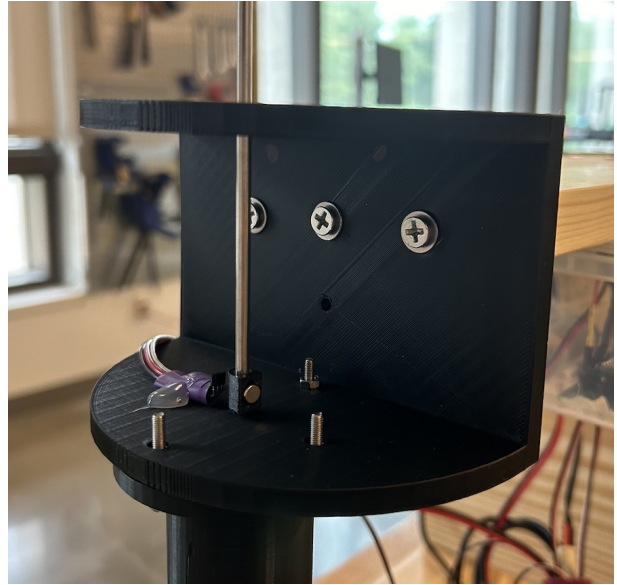
(b) Motor housing 3D printed.
