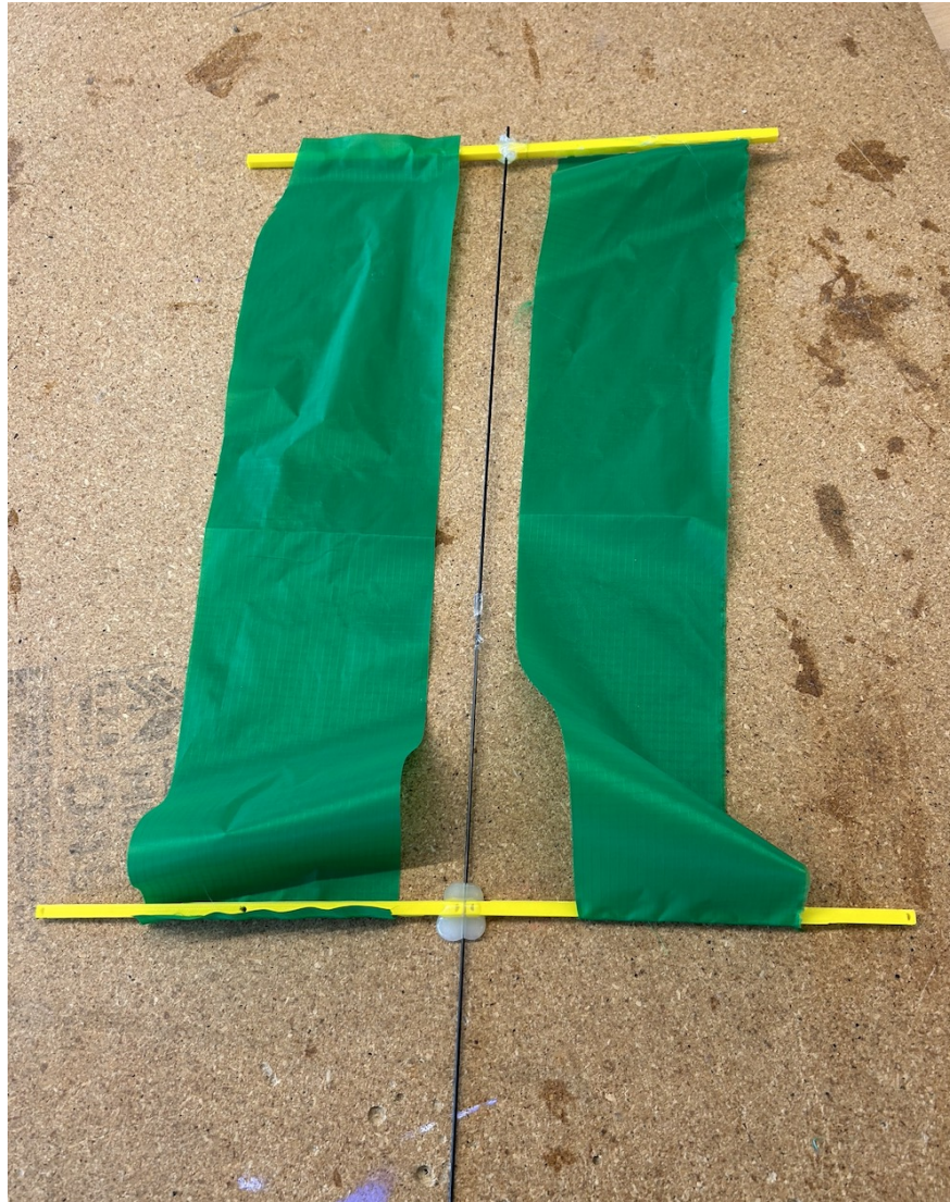
Figure 19: Prototype of lightweight green fabric turbine.
