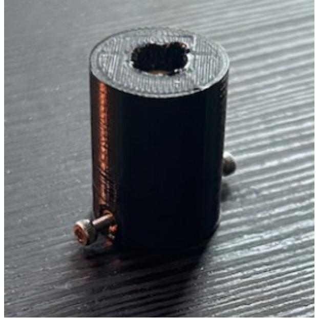
(b) Motor coupler 3D printed with inserts.
