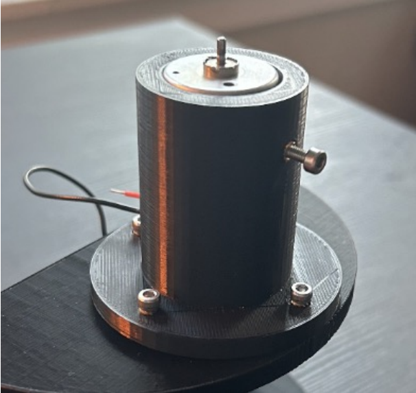
(b) Motor holder 3D printed with inserts.
