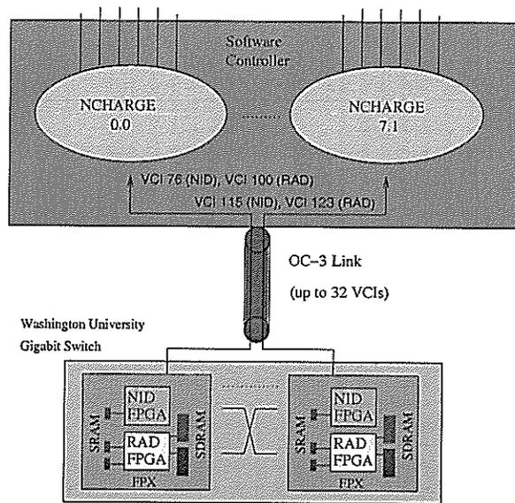
Figure 9: Detail of the hardware and software components that comprise the FPX system. Each FPX is controlled by an NCHARGE software process. The contents of the memories on the FPX modules can be modified by remote processes via the software API to NCHARGE.
