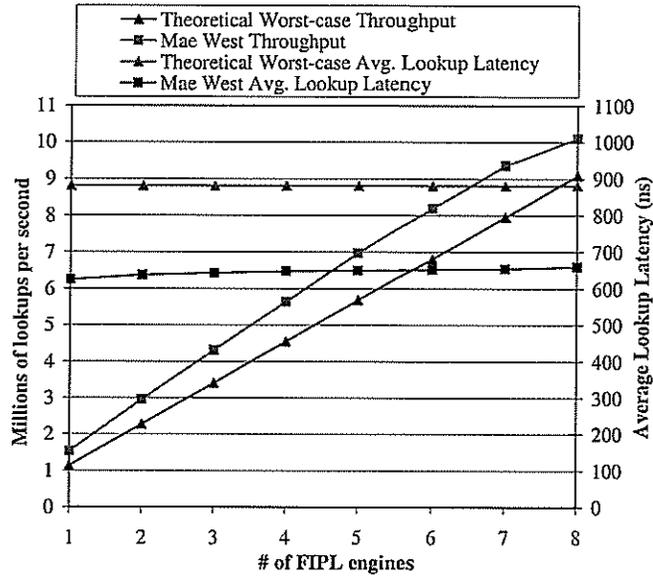
Figure 13: FIPL performance: measurements used a sample database from Mae West on July 12, 2001 consisting of 16,564 routes. Input test vectors consisted of random selections of 2048 IPv4 destination addresses.
