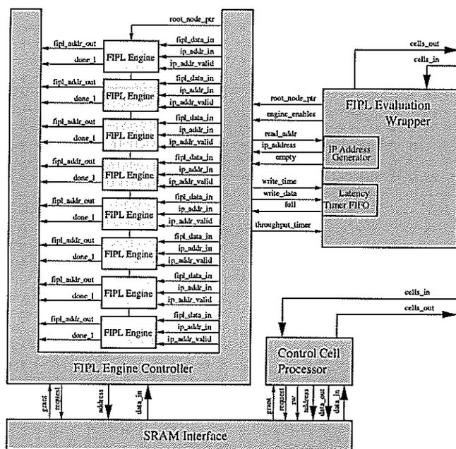
Figure 12: Block diagram of FIPL evaluation environment.
