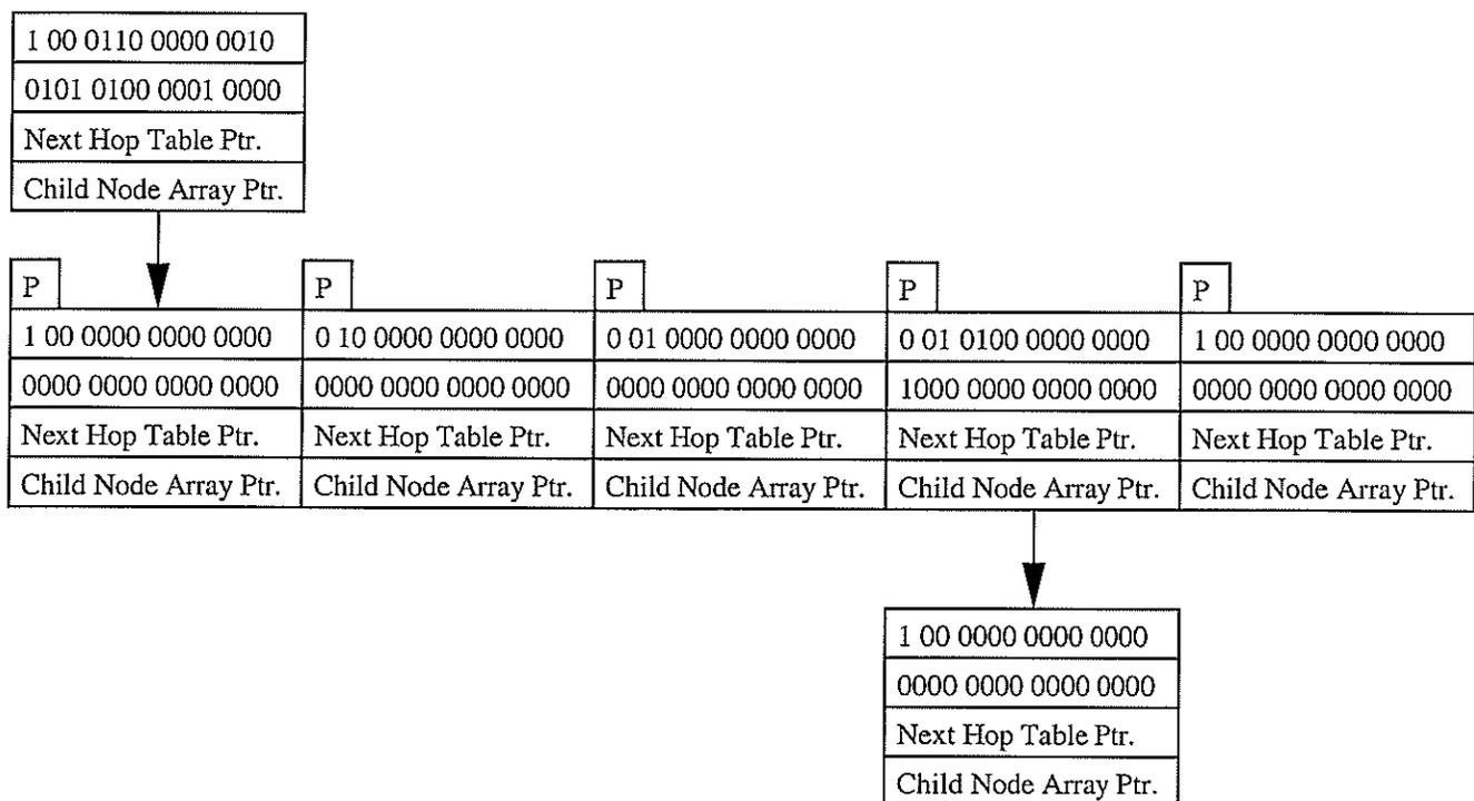
Figure 5: IP lookup table represented as a Tree Bitmap. Child nodes are stored contiguously so that a single pointer and an index may be used to locate any child node in the the data structure.
