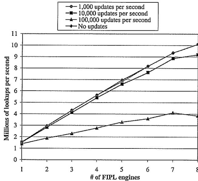
Figure 14: FIPL performance under update load: measurements used a sample database from Mae West on July 12, 2001 consisting of 16,564 routes. Input test vectors consisted of random selections of 2048 IPv4 destination addresses. A single update consisted of a route addition requiring 12 memory writes packed into 3 control cells.
