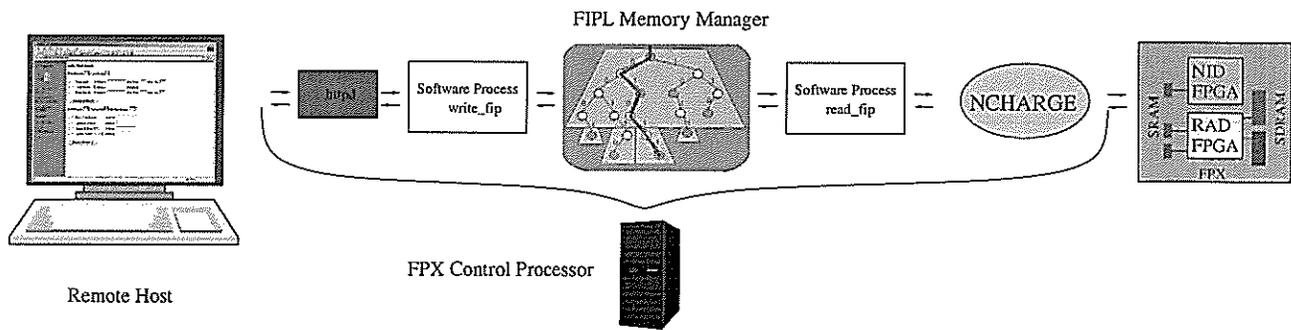
Figure 10: Data flow with FIPL and NCHARGE
