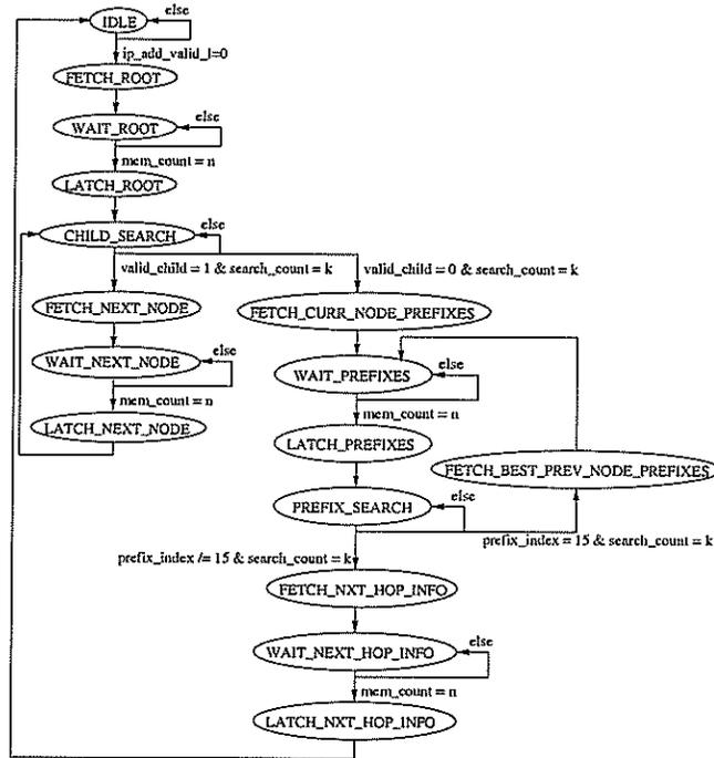
Figure 8: FIPL engine finite-state-machine bubble diagram.
