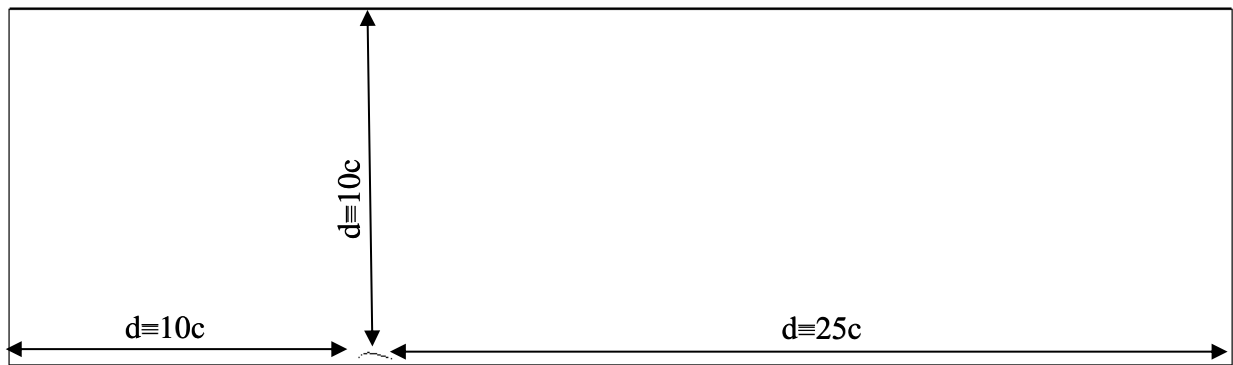
Figure 23. Computational domain around the NACA0012 airfoil with Gurney flap.
