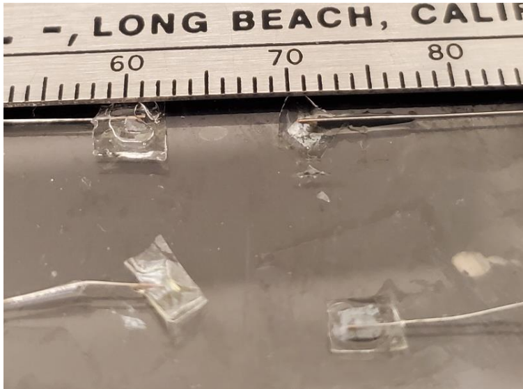
Figure 2 - picture of four prepared antennae. Overall device thickness is ~ 80-200 \mu m. Device width is 3-5mm per side.
