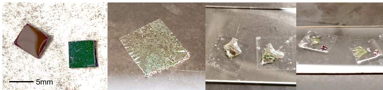
Figure 4 – Photos at select steps of the MoS 2 transfer process. From left to right: 1) two squares cut from the larger wafer, with the green one yet to be lifted off; 2) MoS 2 -PMMA membrane floating in water; 3) two samples recently transferred with water still present; 4) two samples with two layers of MoS 2 transferred and dried.
