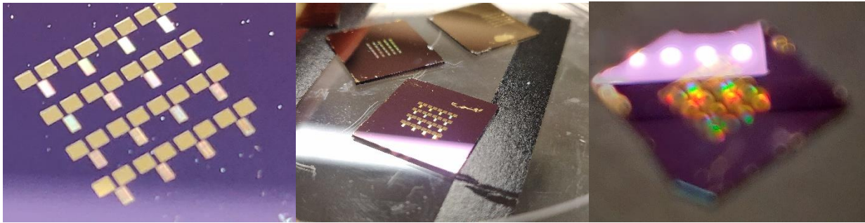
Figure 10 – Images of the IDT patterns on Si-SiO 2 wafers. To the naked eye, the individual digits are not discernible. However, the iridescent diffraction effect they cause is quite noticeable.
