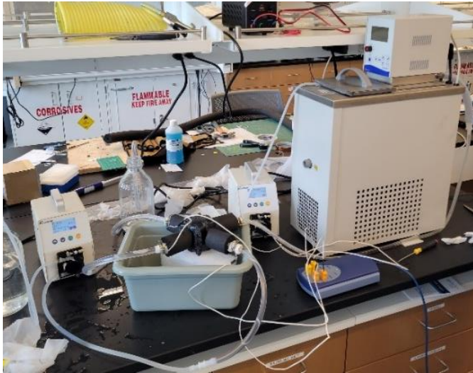
Figure 8: Experimental setup of for the gyroid heat exchanger
