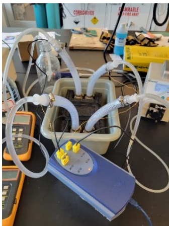
Figure 7: Inlets and outlets of the commercial heat exchangers with thermocouples
