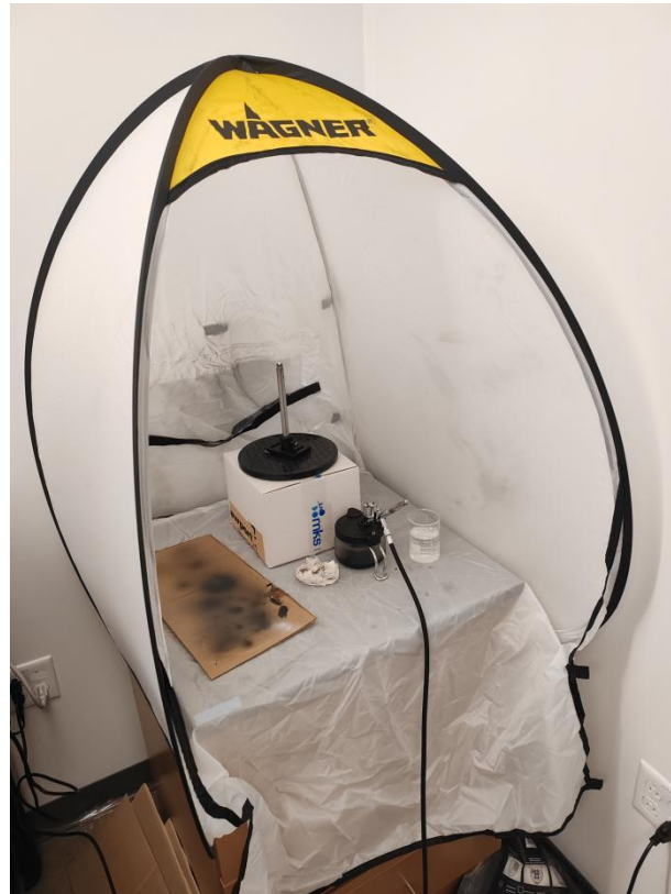
Figure 14. The setup of dyeing to make the speckle pattern on the sample.
