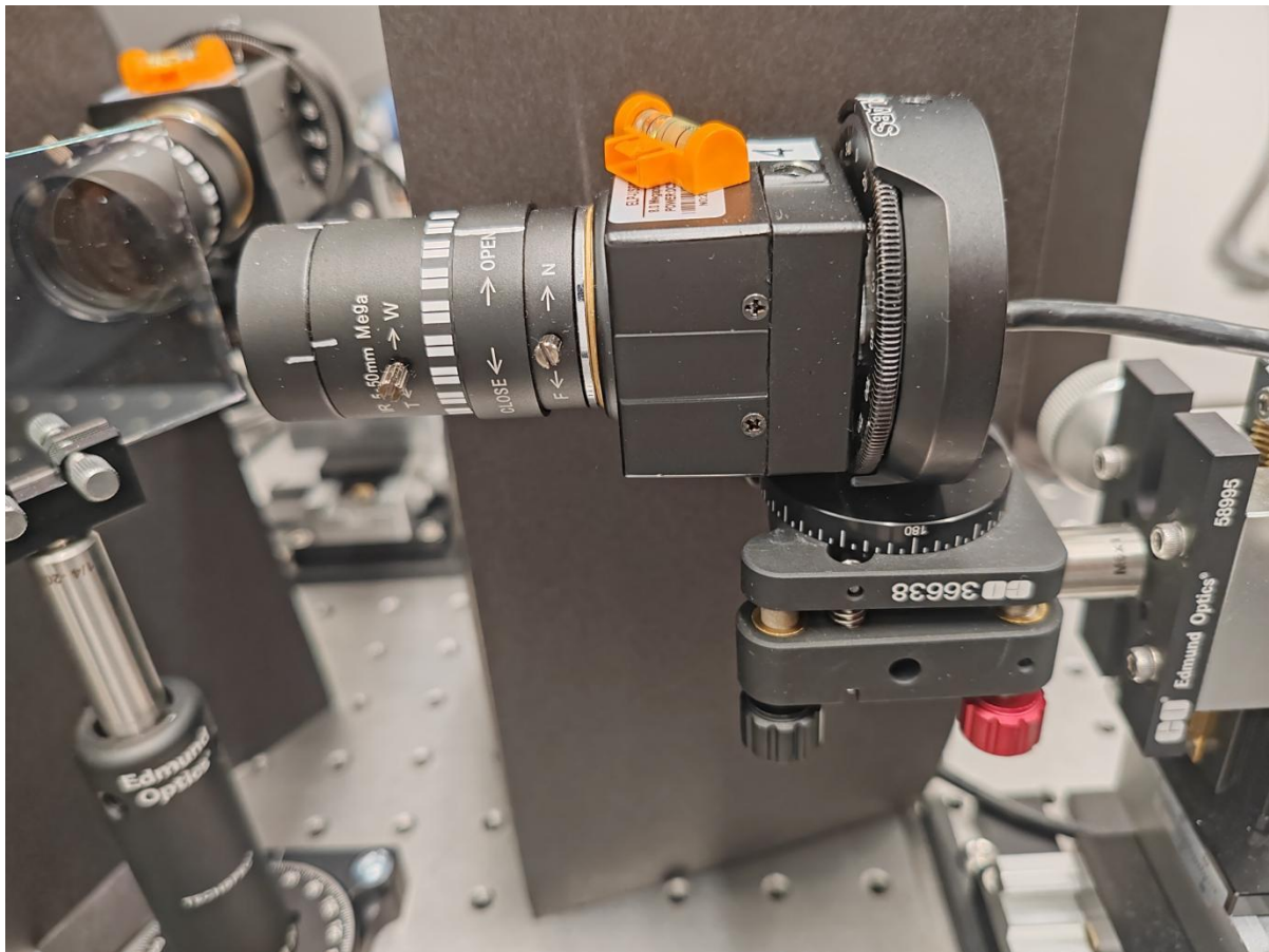
Figure 8. The complete setup for camera 4. The top vertical rotational stage can easily adjust the rotational dislocation and the bottom horizontal rotational stage can easily adjust the horizontal orientation of the camera. Since the left screw of the traditional screw stage can narrowly adjust the vertical orientation of the camera, there is no need to replace it with another rotation stage.
